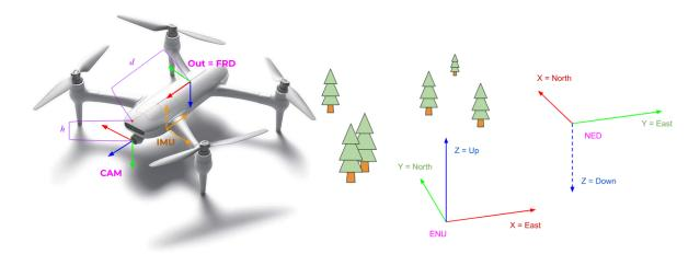
Consider an example, where we have a small UAV with a front-facing camera and we would like to convert from the Spectacular AI GNSS-VIO output poses (IMU-to-ENU) to an FRD-to-NED convention used by, e.g., <u>PX4</u>.
