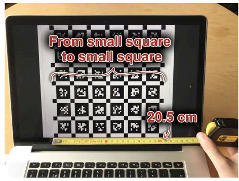
Example: simple AprilGrid calibration using a computer screen: measure and divide by 8.1 to get tagSize.
