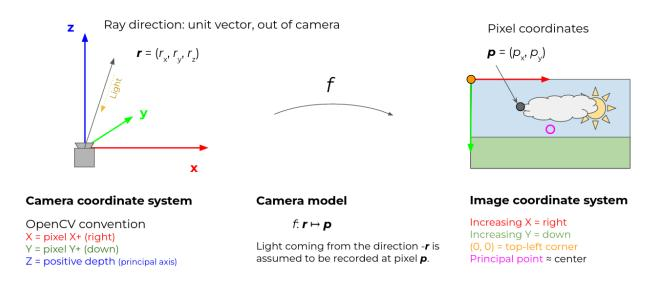
The intrinsic calibration model is a function that maps an outbound ray direction  $\mathbf{r} = (r_x, r_y, r_z)$  to pixel  $\mathbf{p}$ , that is, light coming from the direction opposite to  $\mathbf{r}$  is assumed to be contributing to the pixel with coordinates  $\mathbf{p} = (p_x, p_y)$ .
