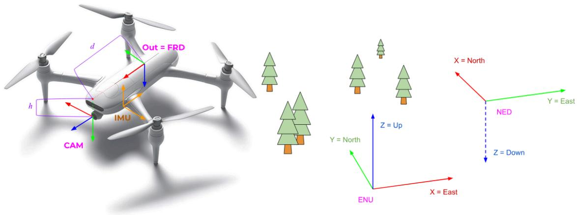
Consider an example, where we have a small UAV with a front-facing camera and we would like to convert from the Spectacular AI GNSS-VIO output poses (IMU-to-ENU) to an FRD-to-NED convention used by, e.g., [PX4](#).
