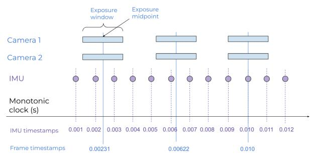
For simplicity, the above figure assumes that the accelerometer and gyroscope are always read simultaneously into one "IMU sample". The example also shows a stereo
