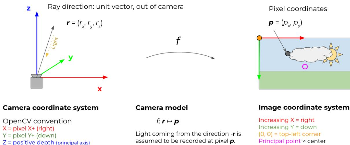
The intrinsic calibration model is a function that maps an outbound ray direction  $\mathbf{r} = (r_x, r_y, r_z)$  to pixel  $\mathbf{p}$ , that is, light coming from the direction opposite to  $\mathbf{r}$  is assumed to be contributing to the pixel with coordinates  $\mathbf{p} = (p_x, p_y)$ .
