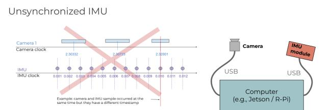
The most common misconfiguration is a system where the IMU and cameras have separate clocks, whose timestamps have no direct relationship. This adds two problems which are very hard to fix in real-time software:
